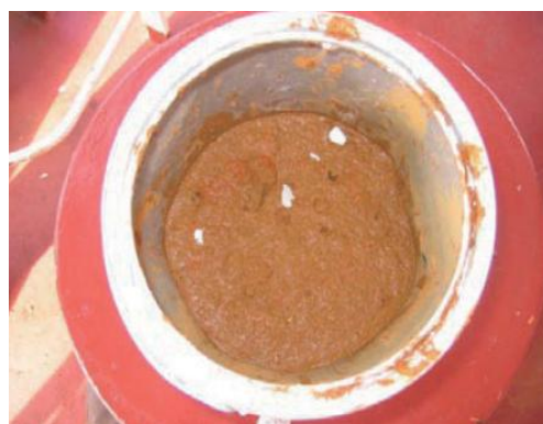
After test(cargo liquefied)
