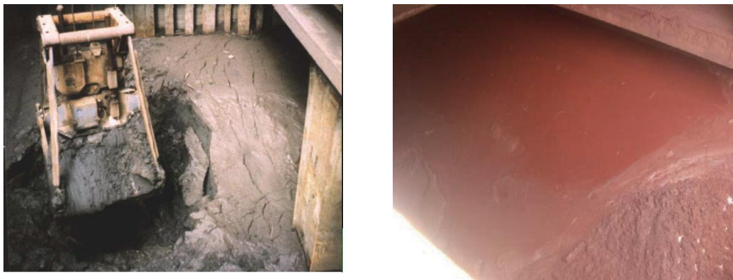
Figure 1 Cargoes liquefied and moisture migration
